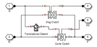
The model implements Dog Clutch, Translational Detent and a modified version of Cone Clutch blocks. Refer to each block reference page for more information on the corresponding block function. You can use a similar approach to model customized versions of the synchronizer. One example is the Transmission (Detailed) subsystem in the model sdl\_vehicle\_manual\_transmission.
