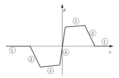
Because the ball is spherical and the notch is symmetric, the horizontal force versus displacement function is symmetric about the origin. (See "Peak Force and Notch Width" on page 1-401.)
