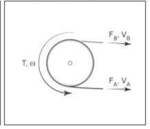
The translational velocities of the two rope ends are functions of the drum radius and angular velocity. Each translational velocity is equal to the tangential velocity of a point at the drum periphery according to the expressions:
